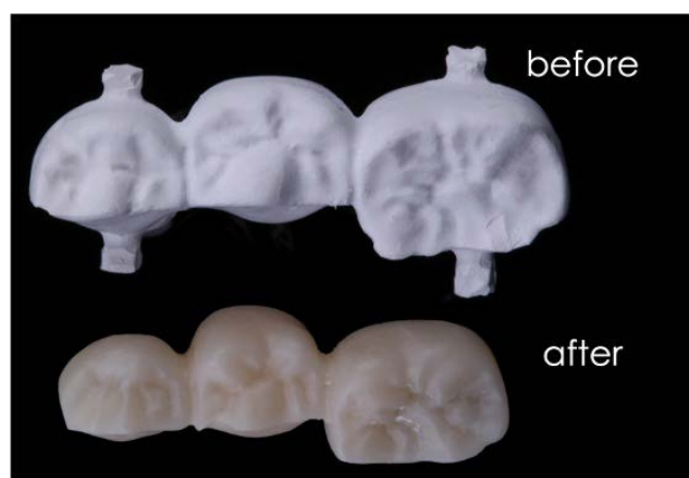
FIGURE 6: Zirconia restoration prior to sintering (above) and after sintering (below)
